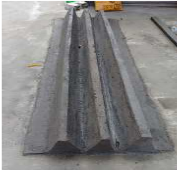
Mould for the construction of roof
