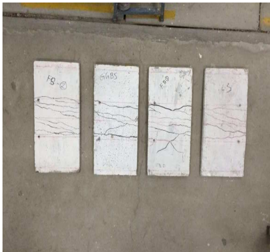
Fig.2 Crack pattern on Ferrocement Slabs
