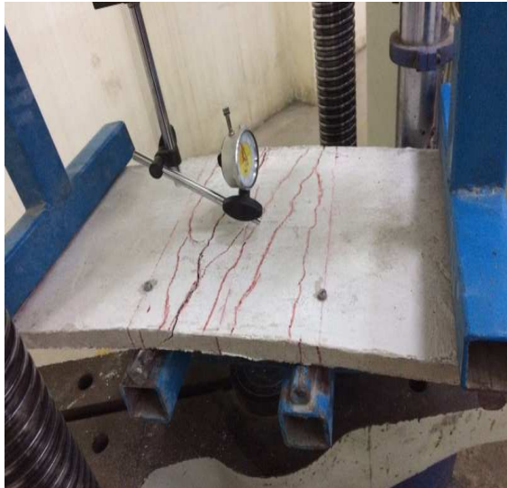
Fig.1 Flexure test on Ferrocement slab
